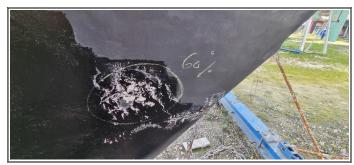
reduced before applying a new gelcoat layer. Proper drying is essential to prevent the trapping of moisture, which could exacerbate the problem over time. After the repair, it is advisable to conduct another moisture meter reading to confirm the effectiveness of the drying process.
